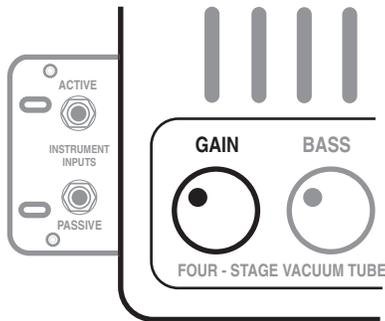
As the **GAIN** control is increased past 12:00 a richer, more “well-rounded” voice becomes dominant and headroom starts to diminish in increments until eventually, a tube overdrive sound appears as the 12AX7 input tube is driven into saturation.
