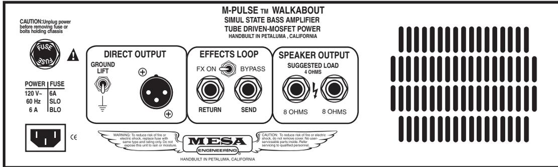
**FUSE:** This is the A.C. Mains Fuse for the *WalkAbout* REPLACE ONLY WITH A SLO-BLO TYPE FUSE OF THE PROPER RATING. THIS IS EXTREMELY IMPORTANT, AS THE *WalkAbout* DRAWS A SUBSTANTIAL AMOUNT OF CURRENT AT HIGH OUTPUT LEVEL SETTINGS.
