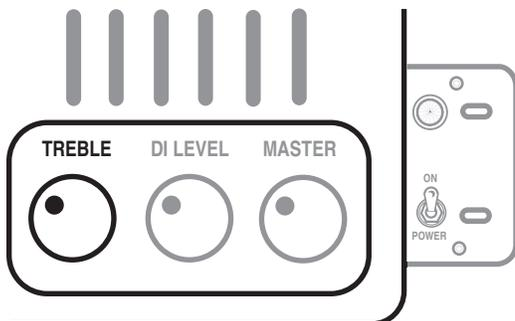
As the control is increased past 12:00, it produces a 6db per octave rise in gain starting at 723Hz until +20db is reached. From this point, gain remains constant at +20db for all frequencies above 723Hz all the way out to 20Khz. This scheme lends a sweetness of sound while retaining all the necessary cut and focus associated with a traditional passive **TREBLE** control.
