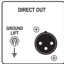
**GROUND LIFT:** This switch removes the circuit-to-chassis ground connection from the XLR jack. Leave it in the grounded position (switch down) normally unless you experience a hum when connecting to a console.
