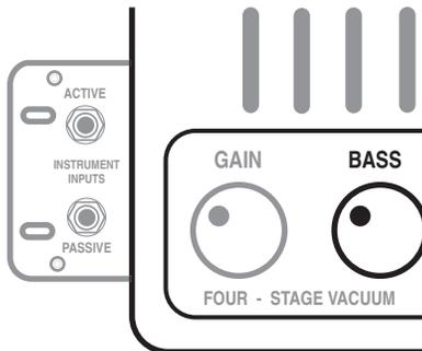
The **BASS** control is actually a gain and frequency control all rolled into one with the Q center at 55Hz and harmonics in both low and high directions are affected because of its broader band nature. As the control is increased past 12:00 there is a 6db per octave rise in gain with the frequency topping out at 321Hz. With 12:00 straight-up representing “flat” (a no boost/no cut setting).
