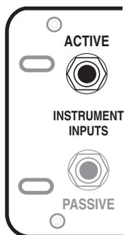
The **ACTIVE** Input is padded down for greater input stage headroom and this works well with basses that use an on-board pre-amp with an active tone control circuit. Usually these instruments put out a much hotter signal than conventional basses, even when their tone controls are set “flat”. The added headroom is needed to prevent clipping in the first stage of the pre-amp and the **ACTIVE** Input should be used whenever instruments that utilize active style pickup/EQ harnesses are used.
