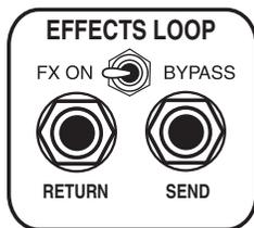
**FX ON / BYPASS:** The **EFFECTS LOOP** circuitry can be completely removed from the signal path with the **FX ON / BYPASS** mini toggle. This removes all associated loop circuitry from the chain and ensures the purest signal path and maximum sonic performance when outboard processing is not being used.
