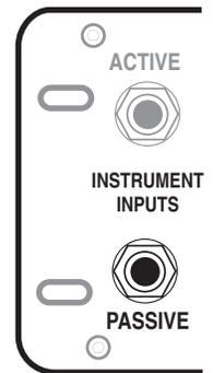
The **PASSIVE** Input is set up for more conventional basses with passive pickups that produce lower output signal levels. This jack is more sensitive than the **ACTIVE** Input and therefore can drive the first stage to clip with a much lower signal. Keep this in mind if you play with a heavy touch or want a little bit of growl or front end clip. In those scenarios this jack can be quite useful to push the first stage of the pre-amp.
