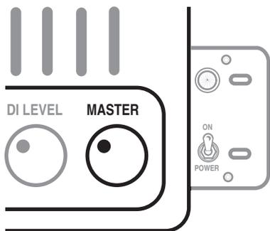
**NOTE:** Use the **MASTER** output level control with care. The *WalkAbout* is capable of very loud output volumes that could potentially cause damage to your hearing or the hearing of others. May we suggest always beginning your set-up by zeroing-out the **MASTER** output level control to avoid accidental volume attacks on unsuspecting bandmates, engineers or audiences.
