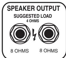
A speaker load of 8 Ohms may also be used though the overall power will be reduced to roughly 150 watts using this rate of impedance.
