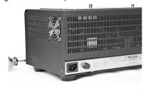
**Caution:** There are three pairs of wires connecting the chassis to the cover. **Do not** lift the cover straight up. With the rear of the amplifier facing toward you, carefully lift the cover and tilt to the left maintaining close distance between the chassis and left side of the cover.
