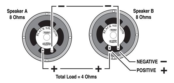
COMBINATION OF SERIES & PARALLEL: This is really just two sets of Series wired speakers connected in Parallel. This is how you maintain a consistent load with multiple speakers. The importance of this is more evident when you have more than one
