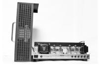
After completing tube maintenance, reverse the above steps to replace the cover. Be sure the wires on the left side of the chassis are tucked in and not pinched between the cover and the chassis as you slide the cover back into place.
