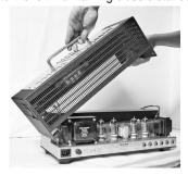
Once the cover is free from chassis, carefully rest the cover on its left side. As an extra precaution, you may place the feet of the amplifier on the cover to keep it from tipping over and pulling out the connecting wires (see close-up photo below).
