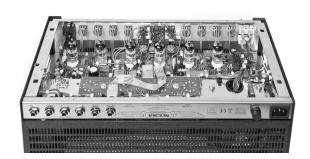
Bottom panel removed for preamp tube maintenance.
