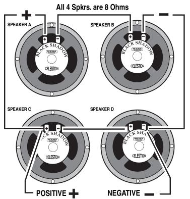
cabinet to connect to your amplifier. This is when you need to figure out the loads and how to wire them up without applying too low of a resistance on the amplifier.
