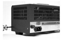
**Caution:** There are two wires connecting the chassis to the cover. **Do not** lift the cover straight up. Carefully rotate the cover forward maintaining close distance between the chassis and front of the cover.
