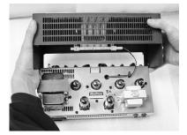
Once the cover is free from chassis, carefully rest the cover on it's top directly in front of the amplifier. As a convenience, you may remove the wire from the LED strip attached to the cover (see close-up photo below) by unplugging it. This will allow you to remove the cover from your workspace.
