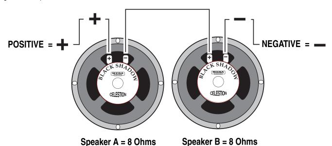
SERIES: Connect the Negative side of Speaker A to the Positive side of Speaker B
