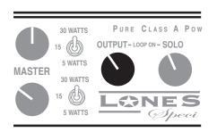
**NOTE:** To use the Lone Star Special amplifier as a power amp - use the EFFECTS RETURN as an input. The SOLO control can be used to attain a footswitchable boost if the Footswitch is connected. It is wired in parallel to the OUTPUT control and therefore also controls the volume of the power section.
