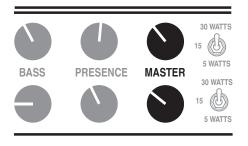
tremely different sound styles and gain signatures. The MASTER control makes possible a wide range of sounds through its ability to use very low Gain sounds at high volumes and conversely, high Gain sounds at low volumes and everywhere between.
