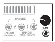
the speaker jacks and is much too strong a signal to connect to the input of a console. Also there is no roll off of high frequencies or shaping, as the speaker does this, so the sound would be less than desirable for recording applications. Should you need a direct recording sound, check out one of our Rectifier Recording Preamp's which are designed specifically for this application and has the necessary circuitry to achieve this difficult task with stunning results.
