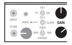
In most guitar amplifiers, and especially in all-tube circuits, the **GAIN** control is the most powerful control in the preamp. It shapes the overall style and character of the sound and is responsible for whether the sound is clean, overdriven or anywhere in between. In your **Lone Star Special** the **GAIN** control is even more powerful. It not only determines the amount of drive, but also acts as an integral part of the tone control string as well.
