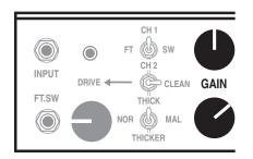
**High (2:15 - 5:00)** Saturates the signal, enhances and expands low and low mid frequencies. While this region provides the maximum saturation and therefor sustain, it also compresses and softens the attack characteristics. For this reason we suggest using this higher region of the **GAIN** control sparingly and only when maximum sustain is needed.
