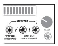
will be achieved for the 15 and 5 watt selections and a slight mismatch will occur in the 30 watt setting where maximum power will be about 30 watts. Using the OPTIONAL jack will produce a correct match for the 30 watt selection boosting overall power to about 35 watts and producing a slight mismatch in the 15 and 5 watt settings (which is fine and may be preferable) giving all three selections a little more punch in the midrange frequencies.
