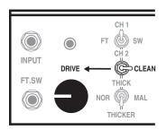
Set to **CLEAN**, all overdrive circuitry is removed and Channel 2 is a slightly higher gain clone of Channel 1. Because of this additional gain in what is otherwise a "rhythm" circuit, Channel 2 is an amazing solo channel for Roots style rhythm work or howling blues solo sounds.
