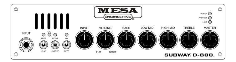
This jack is the instrument INPUT that feeds the first stage monolithic J-FET buffer amp of the SUBWAY D-800. The input sensitivity of this input buffer amp is adjustable with the ACTIVE/PASSIVE switch, the ACTIVE position being about 10dB less sensitive (lower gain) than the PASSIVE position.
