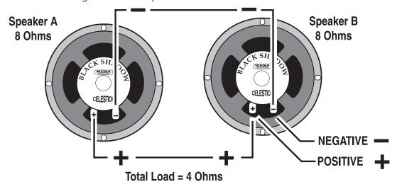
COMBINATION OF SERIES & PARALLEL: This is really just two sets of Series wired speakers connected in Parallel. This is how you maintain a consistent load with multiple speakers. The importance of this is more evident when you have more than one cabinet to connect to your amplifier. This is when you need to figure
